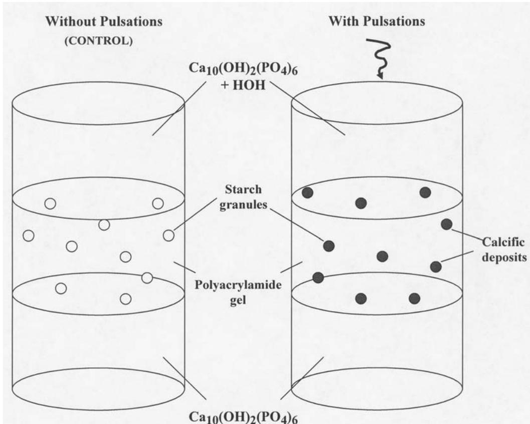
Figure 2. Schematic representation of the *in vitro* experiments using calcium and phosphate ions as mineral markers as deposited by the stress gradients at the polyacrylamide gel-starch granule boundaries induced by the pulsatile forces as predicted by the mathematical model.
