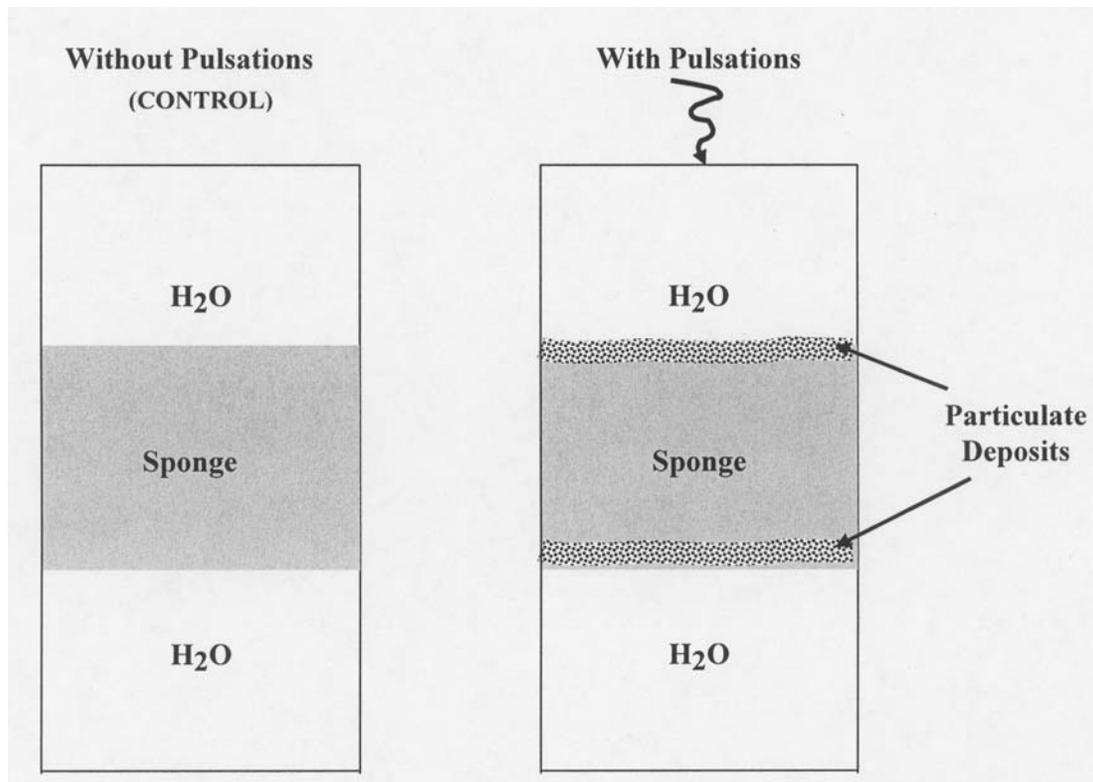
Figure 1. Schematic representation of the *in vitro* experiments using ink-particle markers as deposited by the stress gradients at the water-sponge boundaries induced by the pulsatile forces as predicted by the mathematical model.
