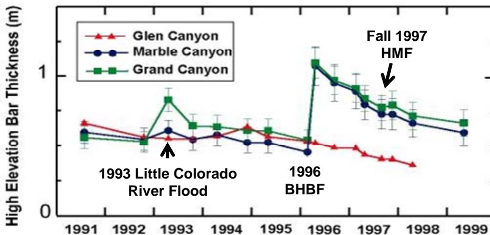
Figure 5. Plot showing changes in sand bar thickness as measured at various locations over time. The effects of various types of floods on the sand bar thickness are illustrated: beach/habitat-building flows (BHBF), habitat maintenance flows (HMF), and the little Colorado River flood was a naturally occurring event in 1993.
